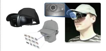
A Near-to-Eye Display (NED) is a way of providing the user with an image that appears to be full-size, despite being physically much smaller. If the NED is integrated with a video-based gaze tracker and a thin see-through screen, it can allow the user to be mobile while still seeing detailed virtual data and images, creating what is essentially a portable heads-up display.
